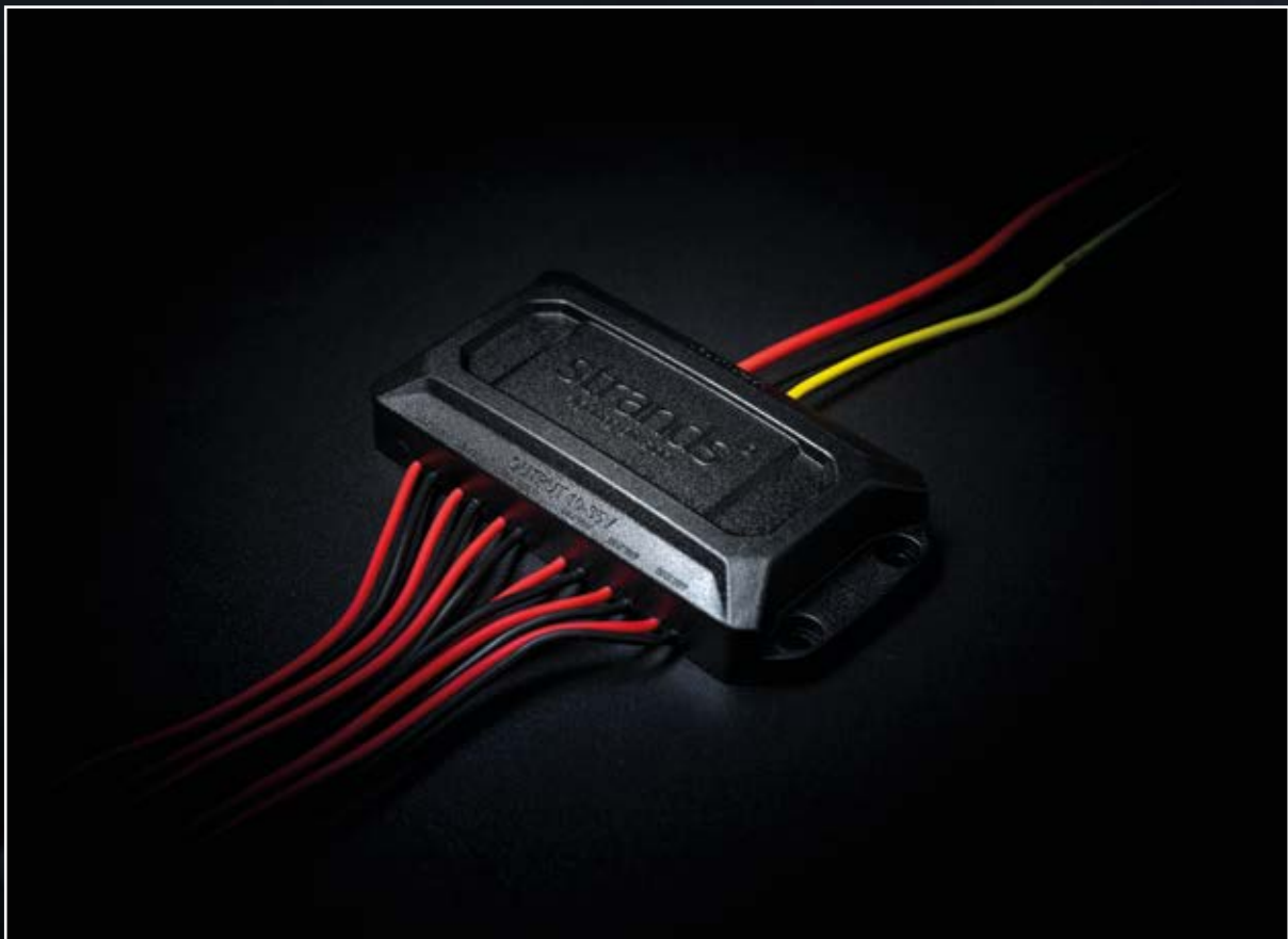
Part No. 270490 CRUISE LIGHT STROBE CONTROLLER
